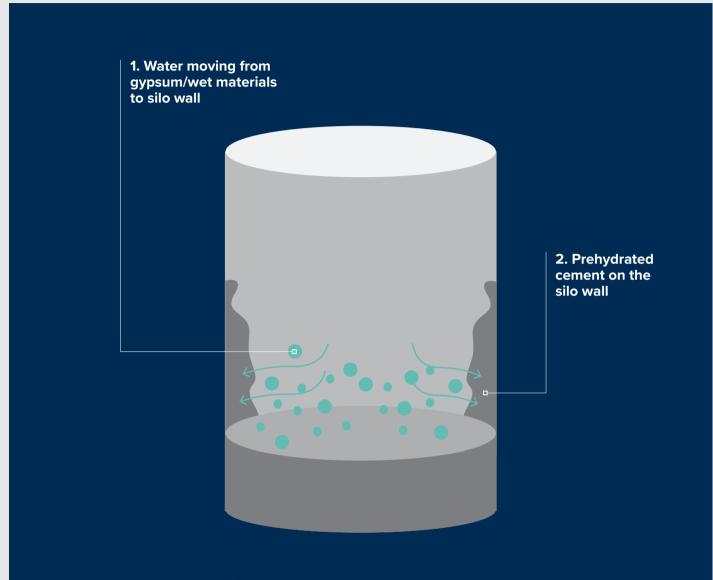
Figure 1. At temperatures above approximately 70°C, the water from gypsum/wet materials moves to the colder parts of the silo (typically the wall, silo outlets and roof), where it prehydrates the cement and eventually forms coating and lumps.
